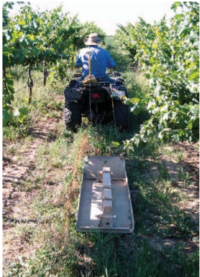
Geonics EM38 instrument being towed on a Perspex sled for on-the-go survey. Photo supplied by Rob Bramley.
